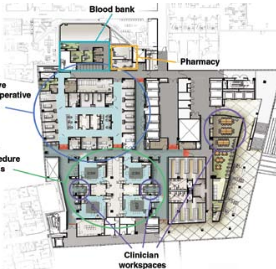
The second floor of the new OR department at Massachusetts General features a 4-OR high-throughput pod. The pod is configured to support parallel processing.
