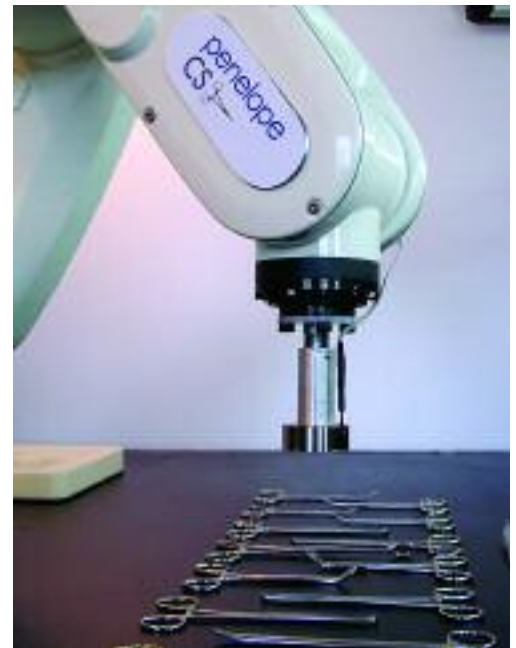
Penelope the robot may be able to assemble and take apart trays.
